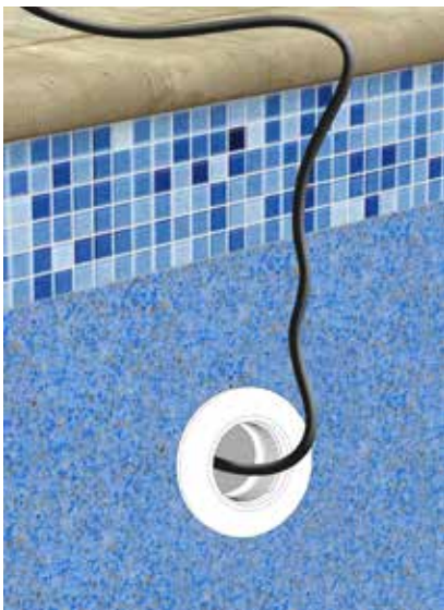
Diag 1. Existing 1½" female thread in pool wall, cable extended to deck.
