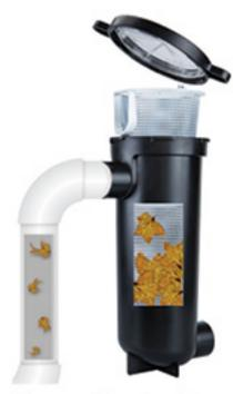
The Abyss canister, simplifies maintenance. Conveniently located by your equipment, the Abyss can be plumbed with multiple canisters to allow for heavier debris environments. Robot cleaners have tiny bags and require you to retrieve the robot from the bottom of the pool many times compared to simply removing the Abyss lid and emptying the basket once.
