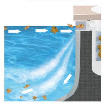
The DownDraft Current uses water in two unique ways. DownDraft both influences submerged debris towards the Debris Removal Drain and it draws floating debris into the mouth of the skimmer. This gives you twice the cleaning power for the same energy dollar making venturi or suction only skimmers obsolete.
