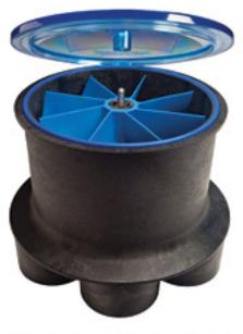
The V360 Water Valve is the heart of the cleaning system. This ultra-efficient valve delivers maximum flow with minimal noise and water pressure variations making it the performance leader in the industry. The Innovative pressure-safe valve design protects your system by ensuring that one port is always open. Large 2" inlet and (6) 2" ports maximizes flow. The see-through lid design allows for inspection of turbine and gear without the need for disassembly.
