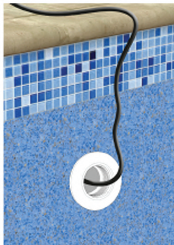
Diag. 1 Existing 1 1/2" female thread in pool wall, cable extended to deck.
