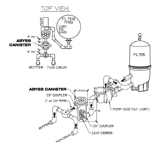
**CAUTION:** The Abyss canister must be plumbed between the pump and any suction side valves in order to prevent excessive water surges and pressures
